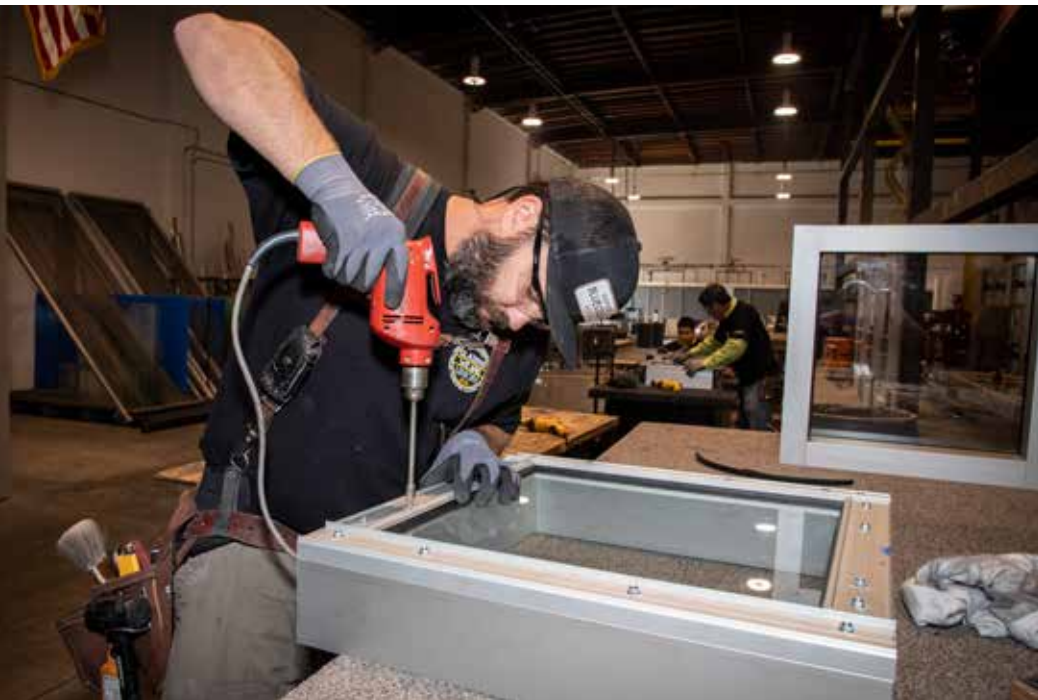
Glazier apprentice Fernando Medina installs pressure bar screws on a curtain wall system.
