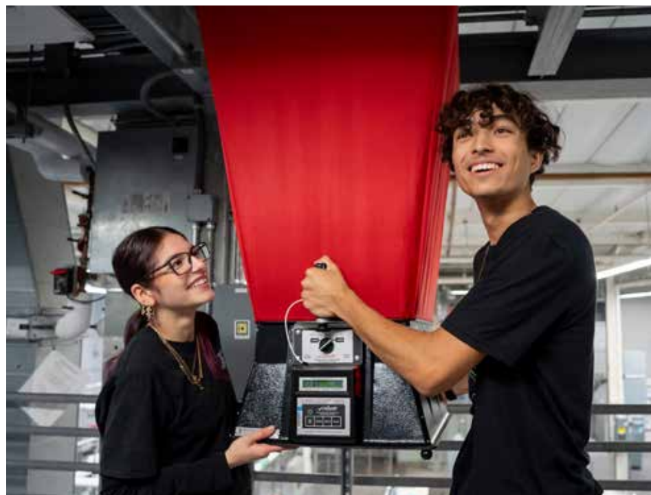
Kayla Rodriguez and Nethaly Urzua with a flow hood, which measures the cubic feet of air coming out of diffusers.
